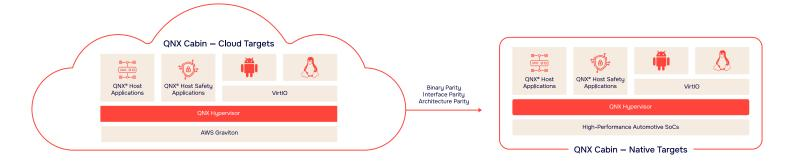
QNX® Cabin for Cloud and QNX® Cabin for SoC are similar platforms, but are aimed at different development targets. This approach means you can start with cloud-based development, then you can move to one of several automotive SoC for further testing and deployment in production.
